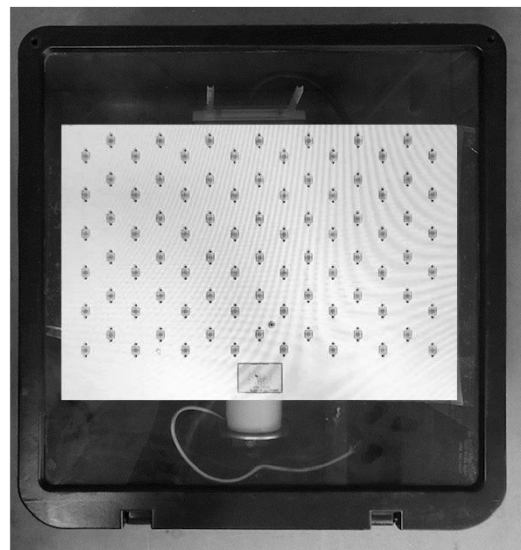
Figure 4 – Cable connected and lens closed
