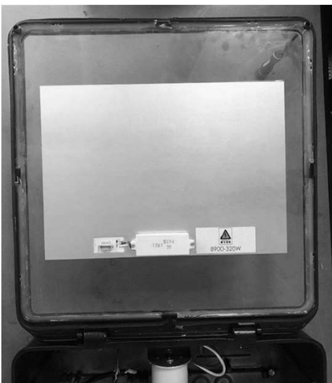
Figure 3 – LED Panel adhered to the inside of the glass lens
