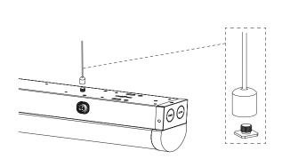
8. Finished aircraft cable installation as shown.
