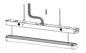
6. Press upward on the cover and lock it.
