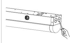
3. Fix the connectiion bracket at the end of one lamp with screw.
