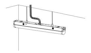
8. To disassemble, push/squeeze both buttons located on opposite ends of the luminaire
