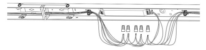
13. The same type of electronic wires are inserted into the same wire nut and combined into a parallel circuit.
