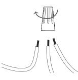
14. Tighten the wires in the wire nut as the photo shows below.
