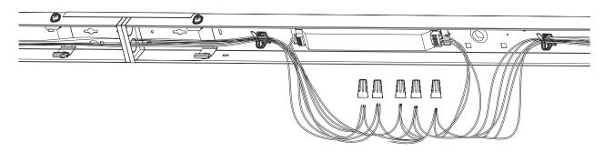
10. The same type of electronic wires are inserted into the same wire nut and combined into a parallel circuit.
