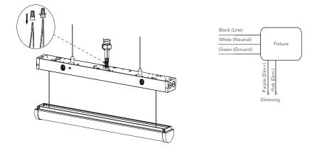
5. Insert the terminal block and wires into the housing.
