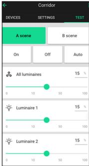
SILVAIR IS A SOFTWARE AND COMMISSIONING APP THAT CONNECTS AND CONTROLS LIGHTING FIXTURES USING BLUETOOTH MESH TECHNOLOGY.
