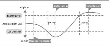
NOTE LUX-OFF SAMPLING TIME - 30S. LUX-ON SAMPLING TIME - 10S. LUX-ON FUNCTION WILL ONLY OPPERATE WITHOUT MOTION WHEN STANDBY IS SET TO +∞.
